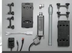
DS-WIFI device is a Wi-Fi modem for long-range wireless data transfer between our data acquisition systems. It is perfectly suited for testing moving objects and for remote measurement applications.
