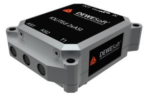
Two analog channels of the device featur anti-alias filtering, A/D conversion and digital filtering. Each of the channels provides precise 5 V excitation for the sensor, which is also used as a reference for the ADC. There is no other internal reference for the ADC, therefore the module should not be used as a general analog input module.
