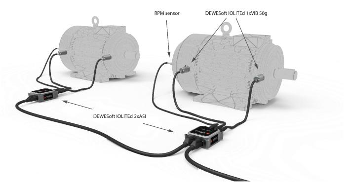
Microprocessor inside the DAQ module transmits the data samples over EtherCAT protocol into DEWESoft software running on a Windows PC, or alternatively to any controller running EtherCAT master on any platform.
