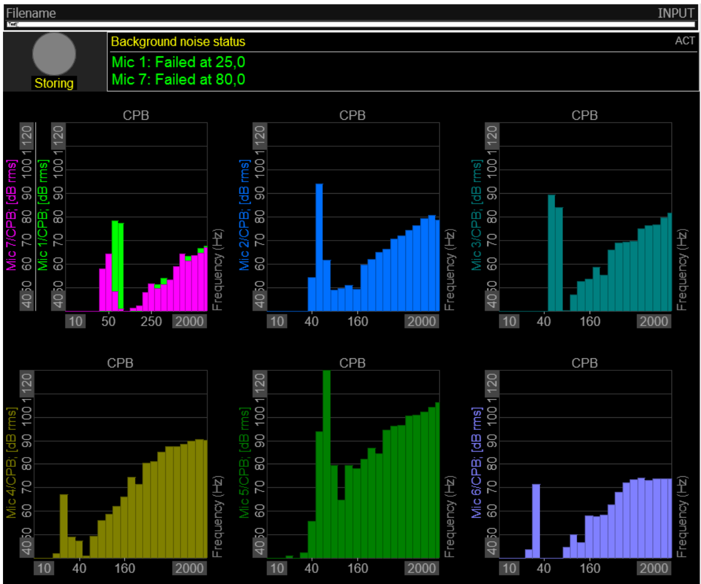
Pre-defined Measure display layout made for the DUT Noise measurement procedure.
