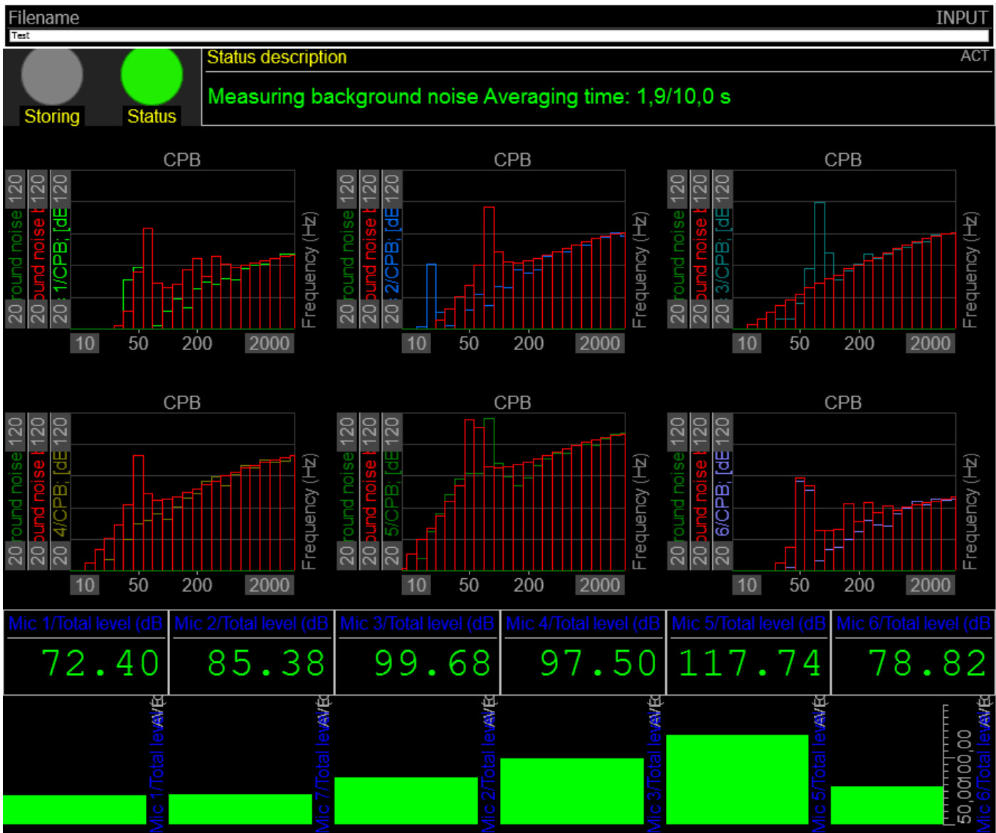
Pre-defined Measure display layout made for the Background noise measurement procedure.
