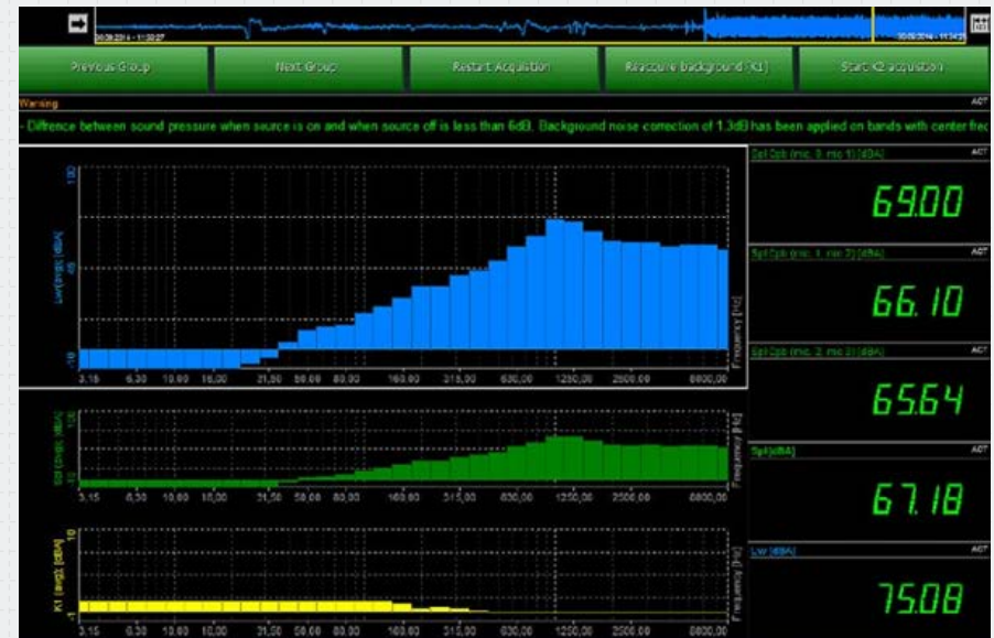
Figure 7. Sound Power measurement in Dewesoft software.
