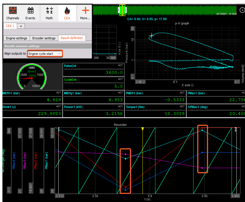
Image 32: Aligning outputs to Engine cycle start
