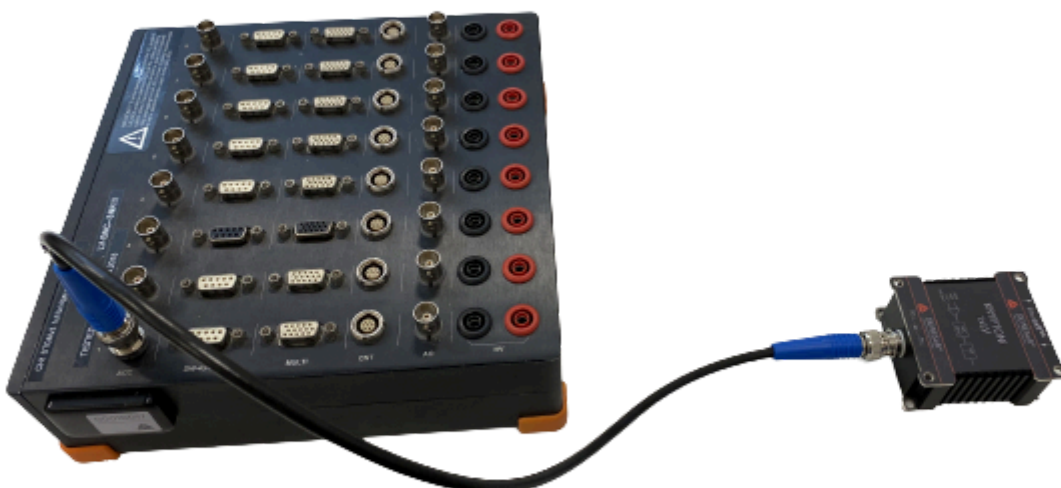
Image: Example of connecting the Kryptoni 1xLV
