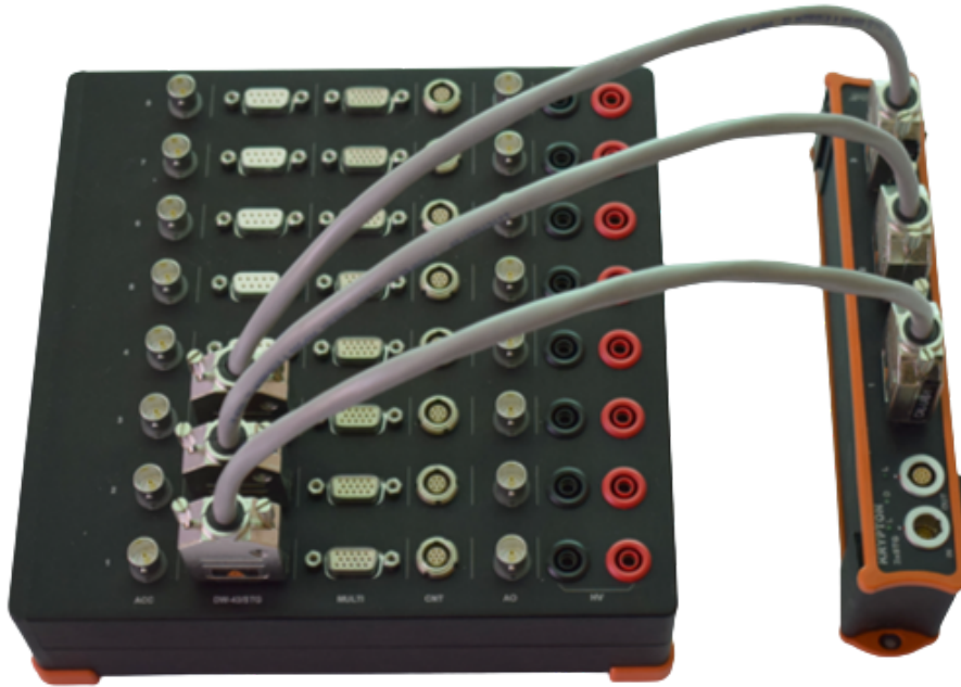
Image: Example of connecting the Krypton 3xSTG channels to the DS-CAL test board
