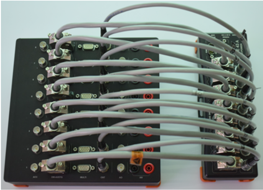
Image: Example of connecting DEWE-43 to the DS-CAL test board
