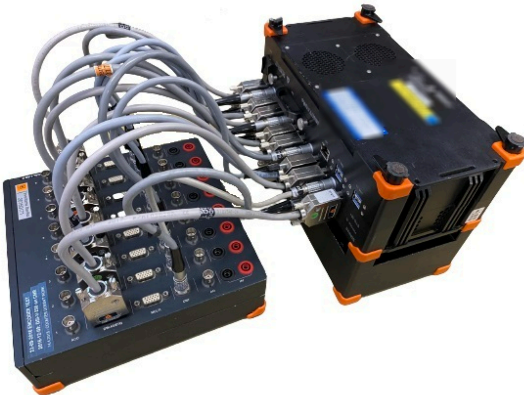
Image: Example of connecting STGM+ modules to the DS-CAL test board
