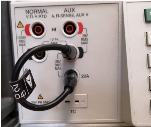
Image: Zero Calibration bridge Fluke 5502E
