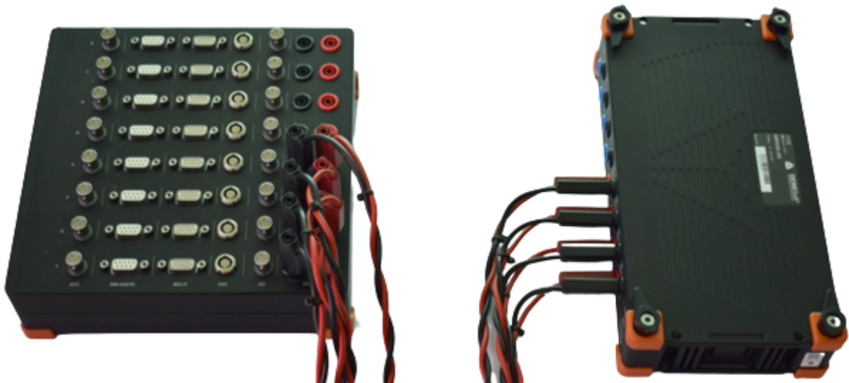
Image: Example of connecting 4xHS-HV Sirius modules to DS-CAL test board
