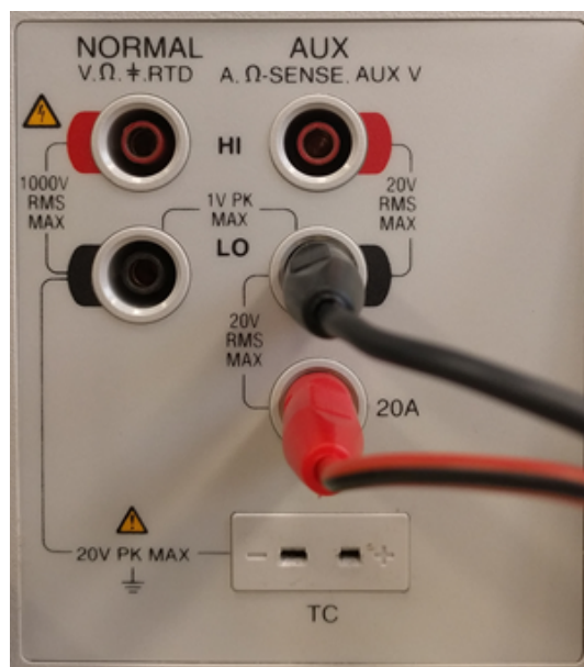
Image: Example of connecting DSI-5A-CAL-CABLE to the FLUKE 5502E multifunction calibrator
