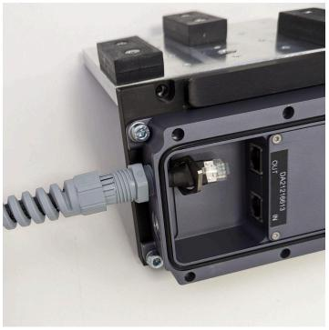
7. Tighten the gland by gripping the nut with a 19 mm wrench. For easier manipulation a specially cut 19 mm wrench should be used.
