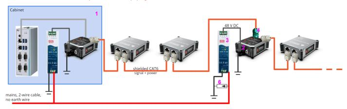
This schematic shows the most recommended wiring in case external power injectors need to be used. The industrial PC, Ethercat power supply and power injector are typically inside the main electrical cabinet (1), together with appropriate surge protection for the power supply system used on installation site (TN or TT).
