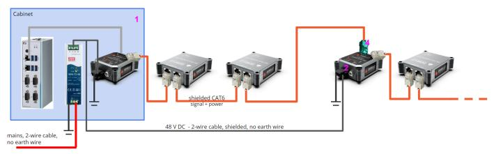
This schematic shows the wiring in case it is not possible to install an external power supply and therefore a 48 V DC power cable is wired to the external power injector.
