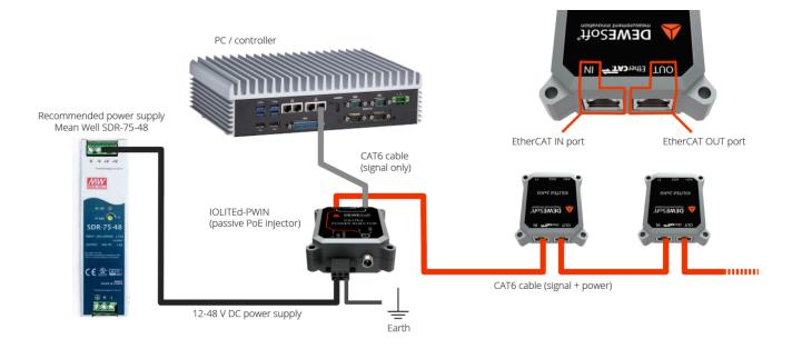
The required power supply: Mean Well SDR-75-48
