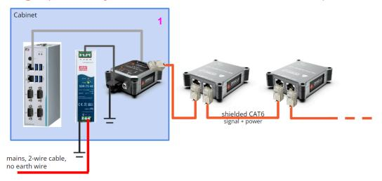
The power supply and power injector should be installed in an electrical cabinet. A single network cable connects the devices outside of the cabinet. The cable shield may be connected at each end of the cables, effectively forming a continuous shield connection along the chain. This is only allowed if the structure to which the devices are mounted is not conductive (i.e. concrete bridge).
