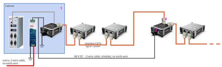
This schematic shows the wiring in case it is not possible to install an external power supply and therefore a 48 V DC power cable is wired to the external power injector.
