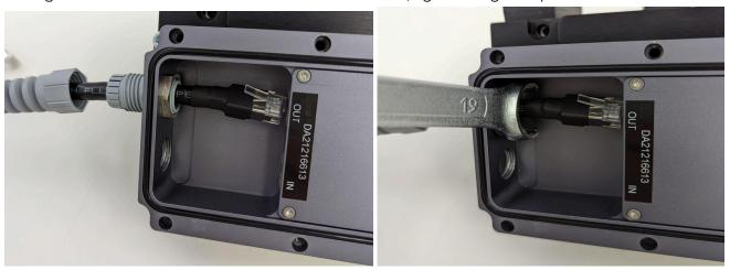
**9.** Plug the RJ45 connector into the RJ45 port of the sensor.
