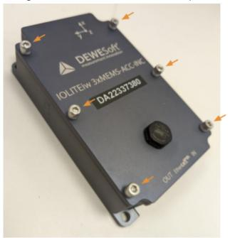
2. There are retaining rings on the screws (see the figure below), so that the screws don't fall out of the holes. However, care still needs to be taken in order not to detach the retaining rings as well. Silica gel capsule is glued to the cover.
