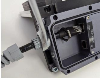
8. Tighten the counter nut on the inside of the device, again using the special 19 mm wrench.
