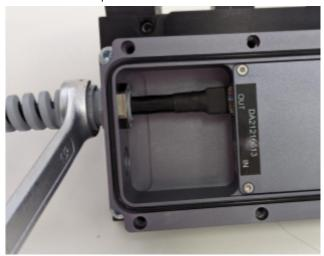
11. A tightened cable gland is shown below.
