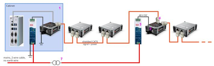
If it is not possible to connect the external power supply and power injector EARTH pins to local earth, there must be an isolation transformer (7) in the MAINS line to the external power supply to protect against electric shock.
