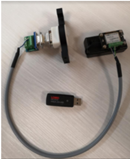
Image 17. WSDA-200-USB & SG-Link-200-OEM connected to a load cell
