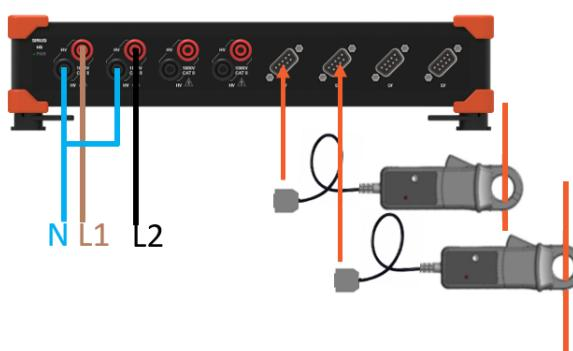
Figure 100. Phase measurement hardware setup
