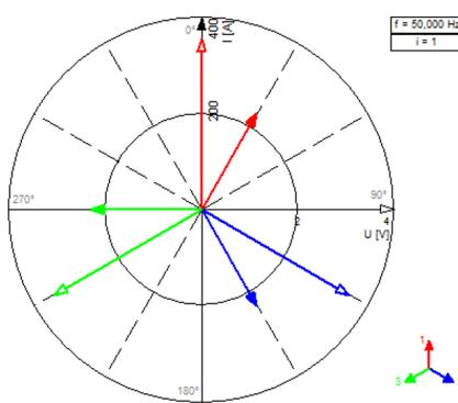
Figure 161. Symmetrical balanced system vectorscope
