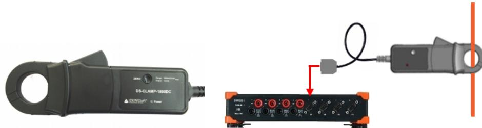
Figure 36. Hall compensated clamp connected to a Surius DAQ
