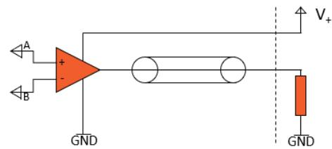
Figure 15. Schematic illustration of a differential voltage probe
