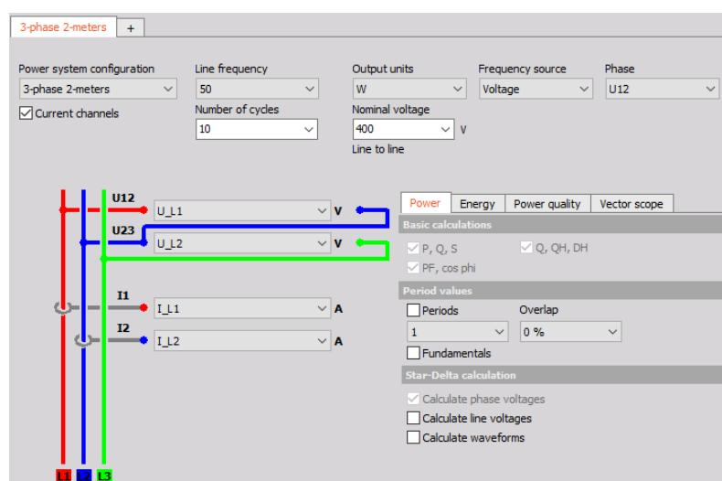
Figure 125. Phase 2-meters power module setup
