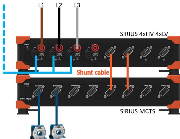
Figure 120. Aron connection hardware setup
