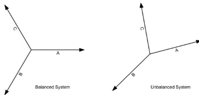
Figure 158. Balanced system and an unbalanced system
