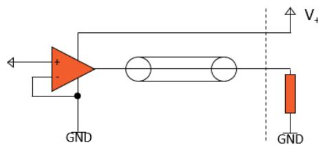
Figure 14. Schematic illustration of an active voltage probe
