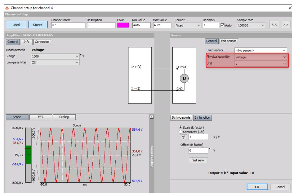
Figure 20. Channel set up screen in DewesoftX®
