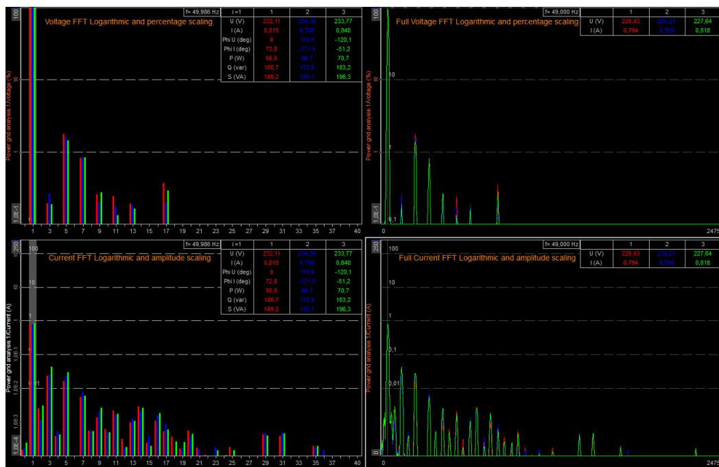
Figure 145. Full FFT display options in the power module
