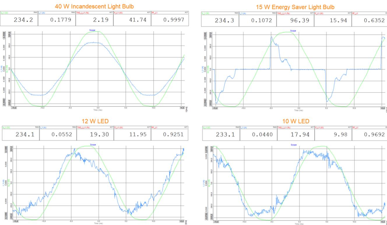
Figure 156. Total harmonic distortion waveform for different light bulbs
