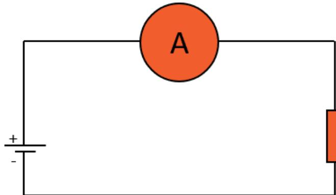
Figure 28. Schematic illustration of connecting an amperemeter
