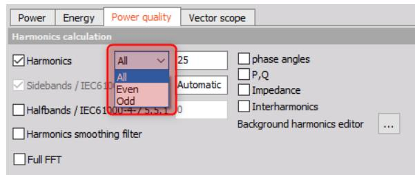
Figure 138. Harmonic measurement calculation options in the power module
