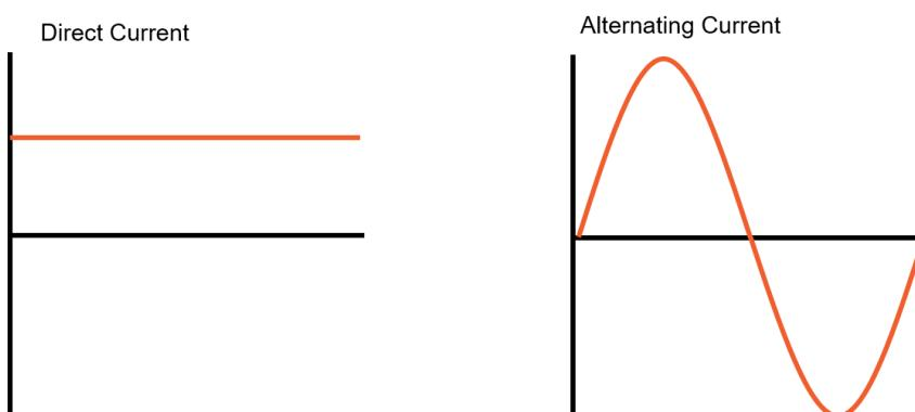
Figure 27. Direct and alternating current
