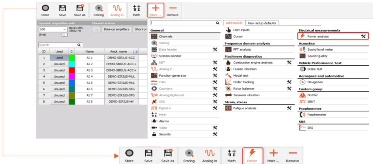
Figure 68. Activating the power module in DewesoftX®
