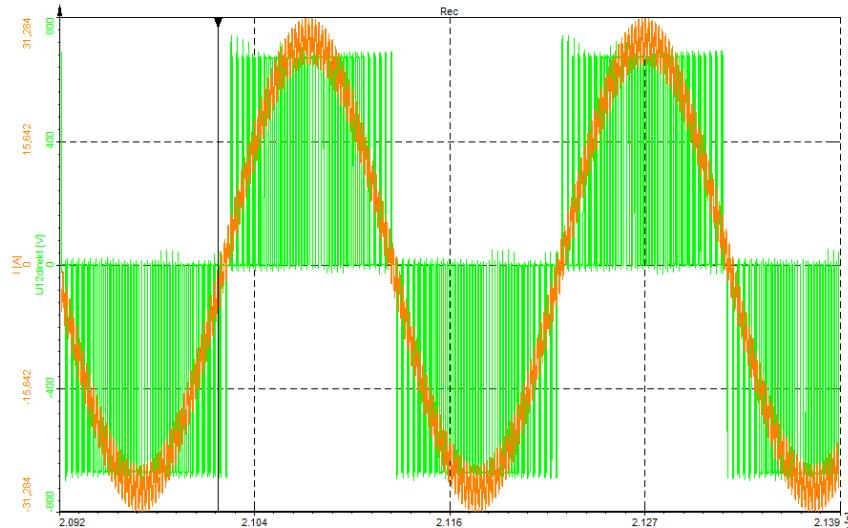
Figure 74. Voltage PWM signal and a sinusoidal current signal
