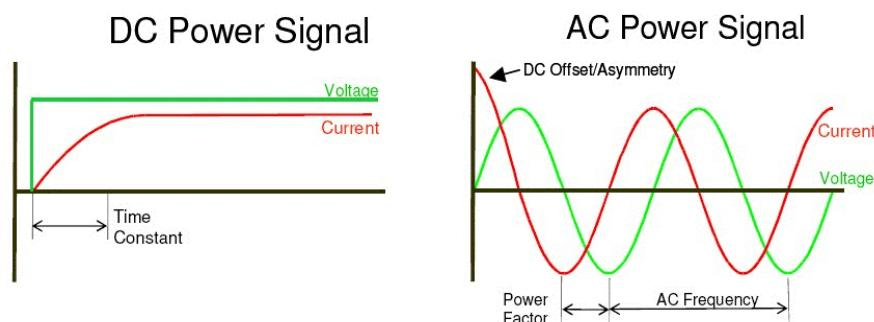
Figure 62. Direct current and alternating current waveforms
