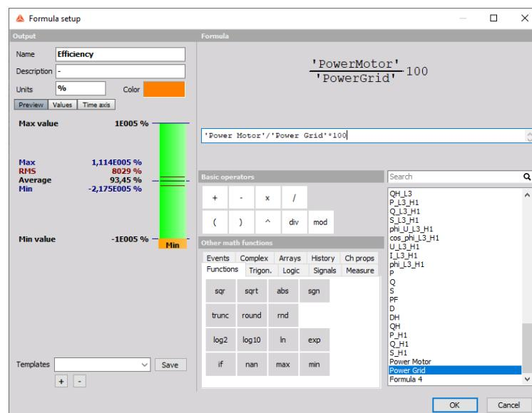
Figure 131. Efficiency calculation in the power module
