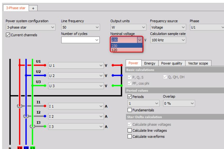
Figure 76. Nominal voltage selection in the power module
