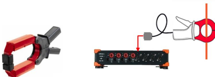
Figure 34. Iron core clamp connected to a Surius DAQ
