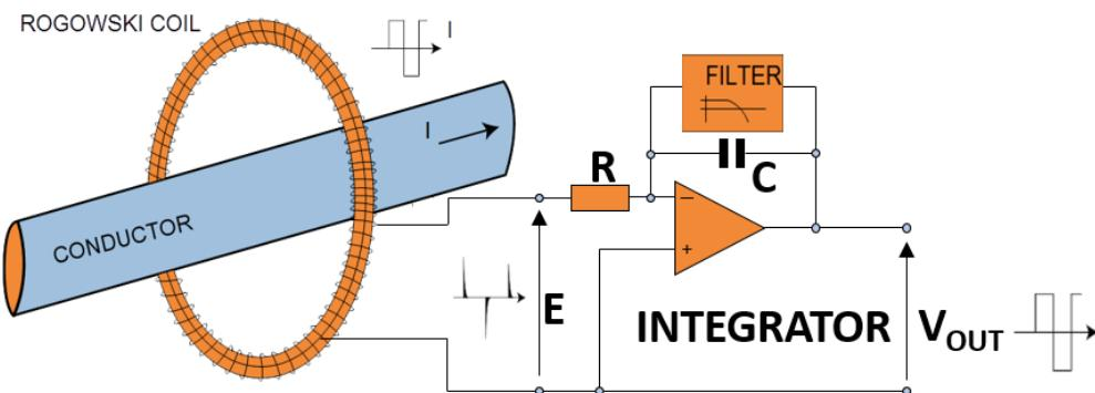
Figure 33. Schematic illustration of the working principle of a Rowgowski coil
