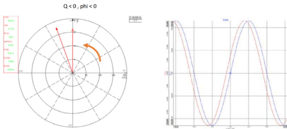
Figure 178. Capacitive current vectorscope and oscilloscope measurement screen
