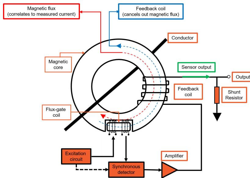
Figure 39. Schematic illustration of the working principle of a Fluxgate clamp
