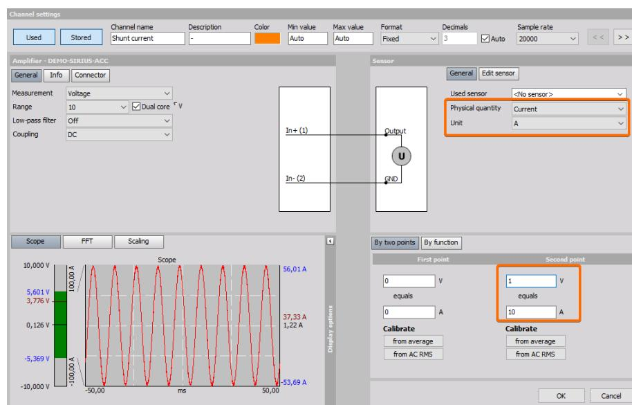
Figure 57. Channel setup for shunt current
