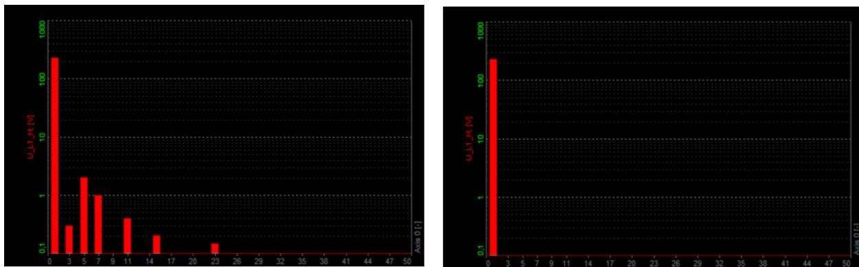
Figure 147. Measurement screen without and with a harmonic filter applied
