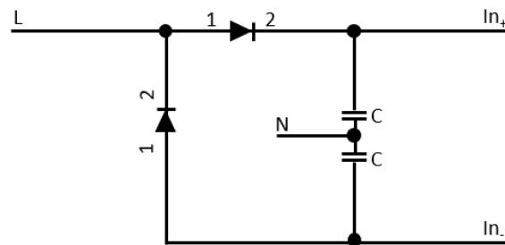
Figure 24. Schematic illustration of a simple voltage measurement on a discharging capacitor
