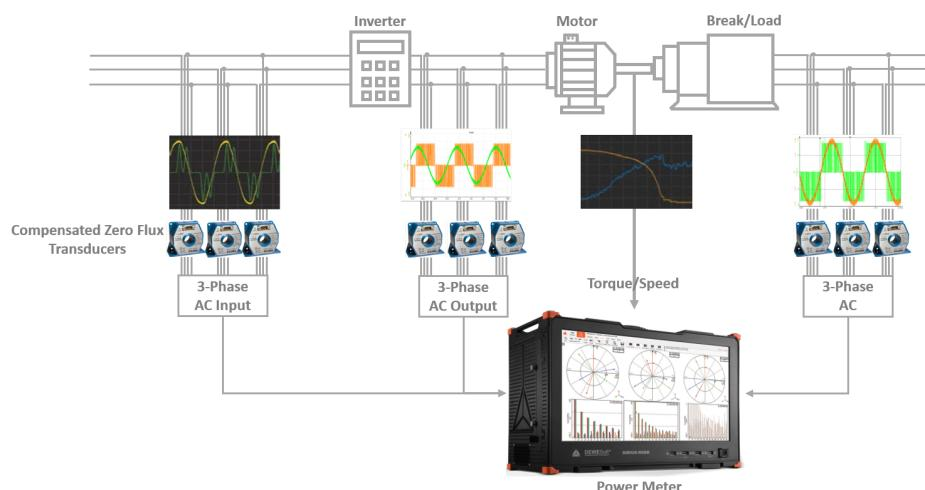
Figure 60. Schematic illustration of a complex 3-phase measurement
