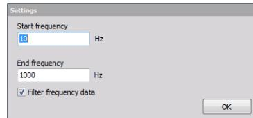
Figure 71. Start and end frequency ranges
