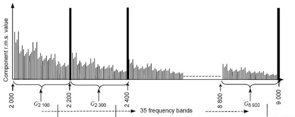
Figure 143. Harmonic grouping according to the IEC 61000-4-7 standard
