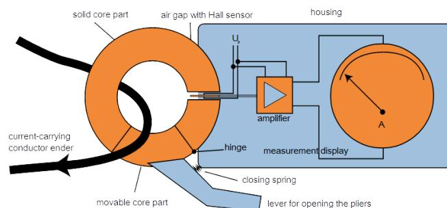
Figure 37. Schematic illustration of the working principle of a Hall compensated clamp
