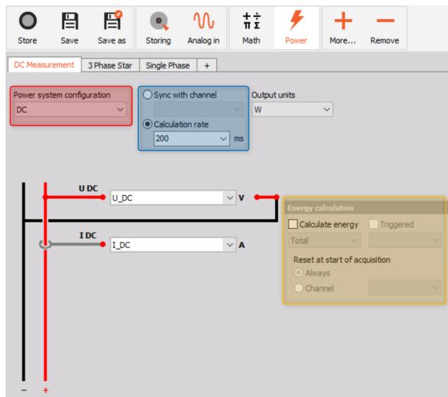
Figure 92. DC measurement power module setup
