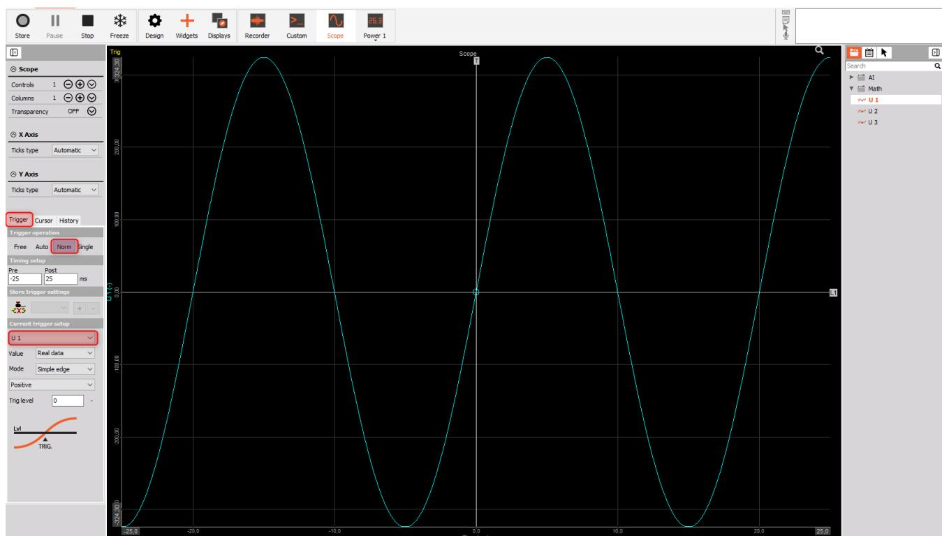
Figure 21. Measurement screen of voltage with a simple trigger
