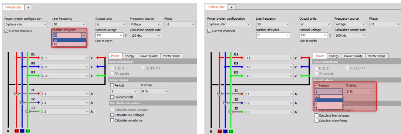
Figure 75. Number of cycles and period values in the power module
