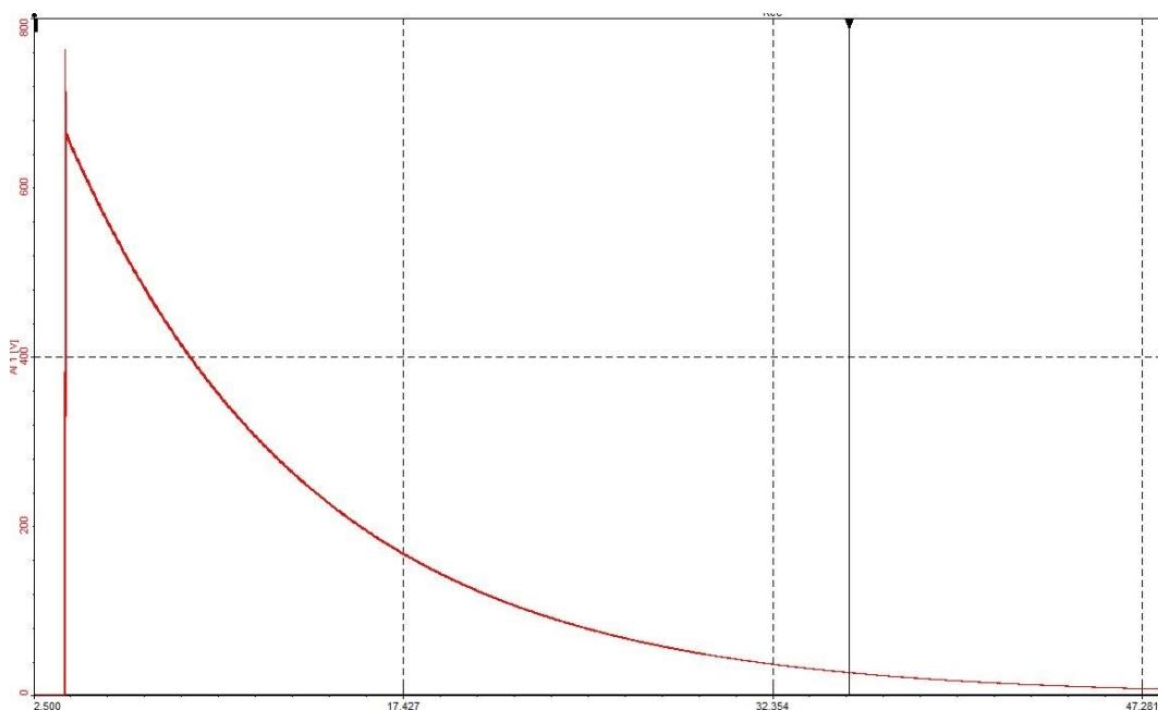
*Figure 25. Capacitor charge and discharge measurement*
