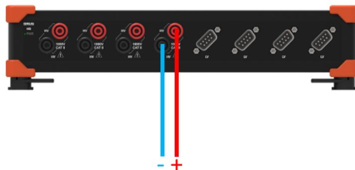
Figure 19. Single phase voltage connection to a Sirius 4xHV 4xLV
