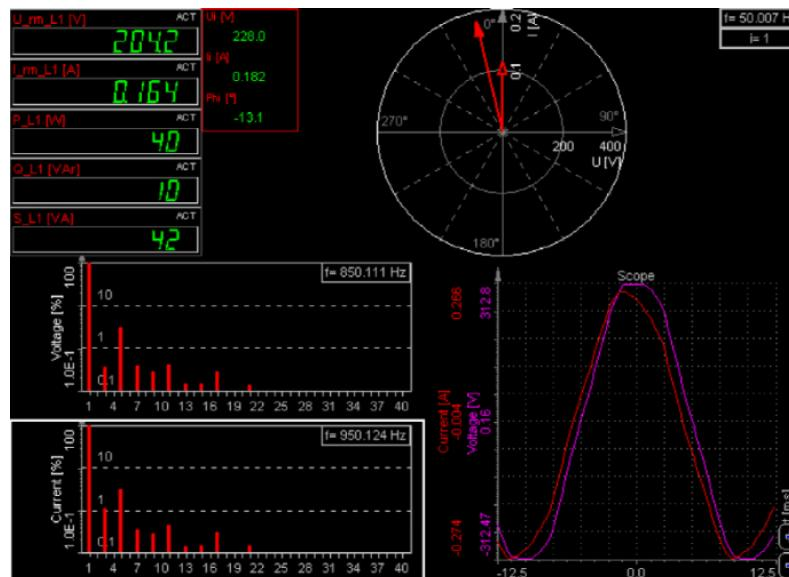
Figure 50. Phase shift caused by a current transducer
