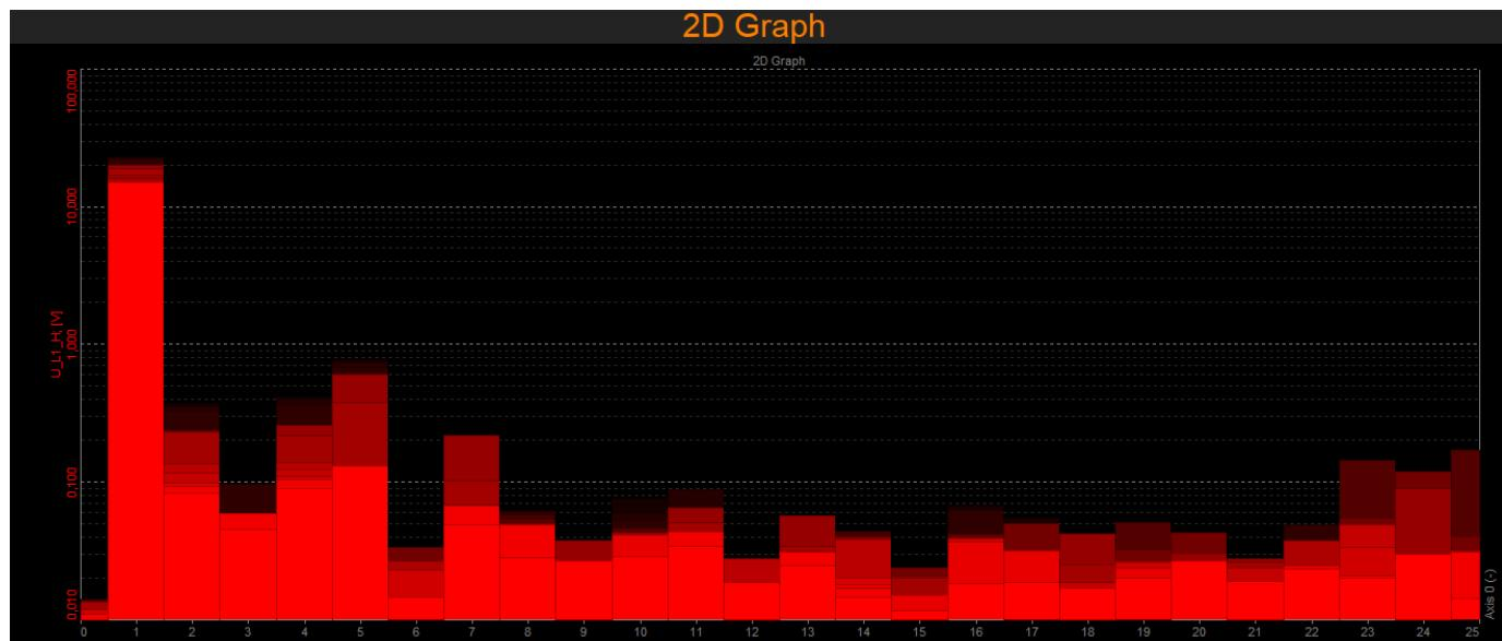
Figure 152. Harmonic 2D graph measurement screen with persistence
