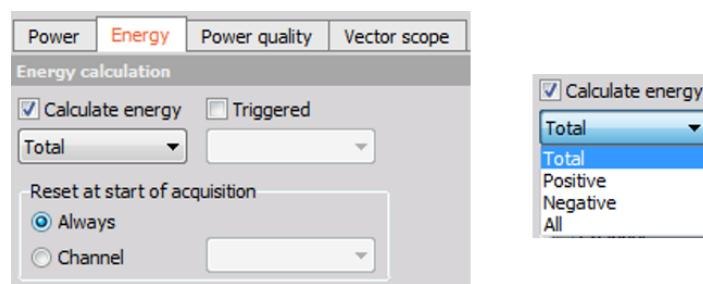
Figure 130. Energy calculations in the power module
