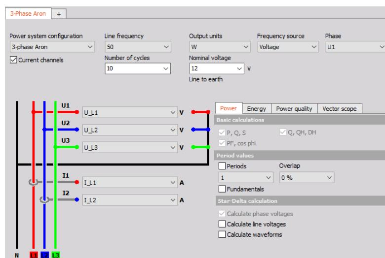
Figure 121. Aron connection power module setup
