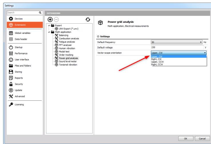
Figure 177. Changing the orientation of the vectorscope in DewesoftX®
