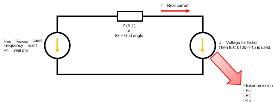
Figure 172. Schematic illustration of the current flicker calculation
