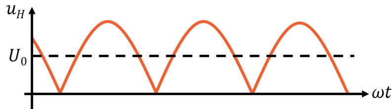
Figure 5. Voltage rectified mean
