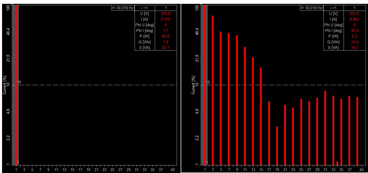
Figure 88. Harmonic FFT view of a pure ohmic load and a non-linear load
