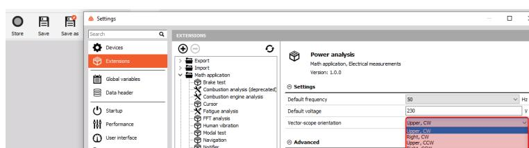
Figure 86. Changing the orientation of the vectorscope in DewesoftX®
