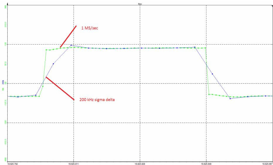
Figure 8. Overshoot of samples which is caused by setting the sample rate too low
