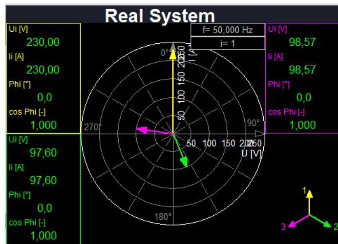
Figure 164. Unbalanced system vectorscope in DewesoftX®
