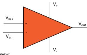
*Figure 7. Schematic illustration of a differential amplifier*
