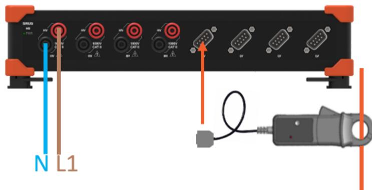
Figure 96. Single phase measurement hardware configuration
