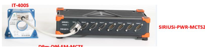
Figure 43. Zero-flux transducer connected to a SIRIUS-PWR-MCTS2
