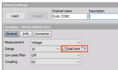
Figure 22. Enabling the dual core mode in DewesoftX®
