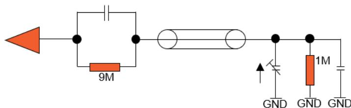
Figure 13. Schematic illustration of a passive voltage probe
