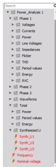
Figure 84. Channel list in the power module
