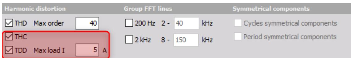
Figure 157. Total harmonic current and Current total demand distortion
