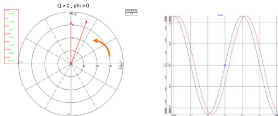
Figure 179. Inductive current vectorscope and oscilloscope measurement screen
