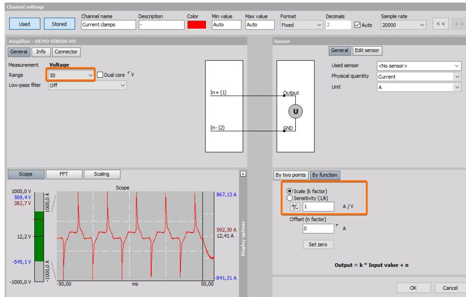
Figure 58. Channel setup for the current clamp
