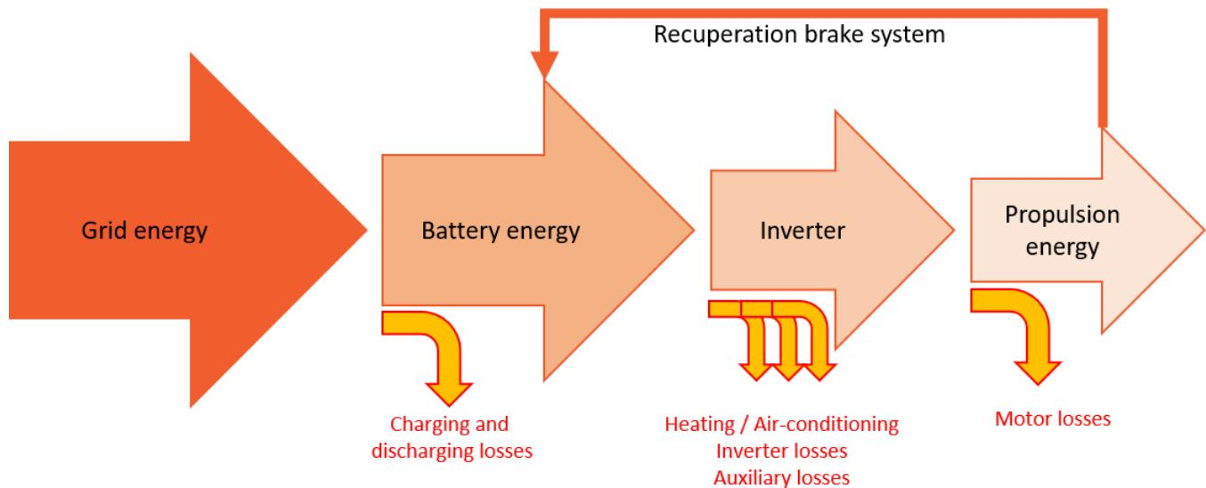
Figure 132. Sankey diagram of an electric vehicle
