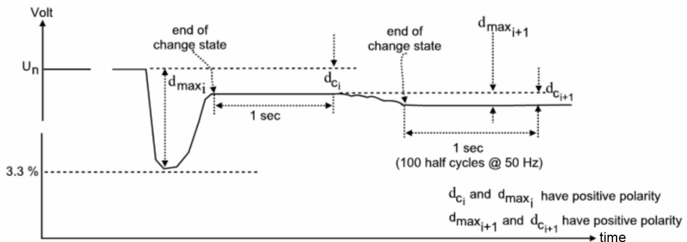
Figure 173. Rapid voltage changes according to the IEC 61000-4-15 standard
