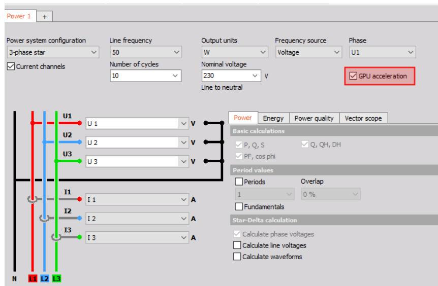
Figure 206. GPU Acceleration in the Power Module
