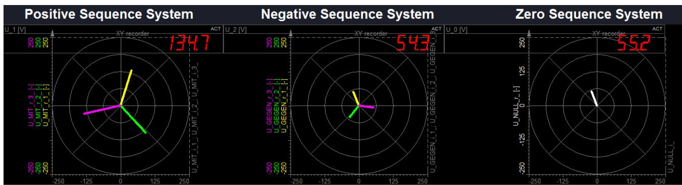
Figure 165. Unbalanced system to balanced system transformation in DewesoftX®
