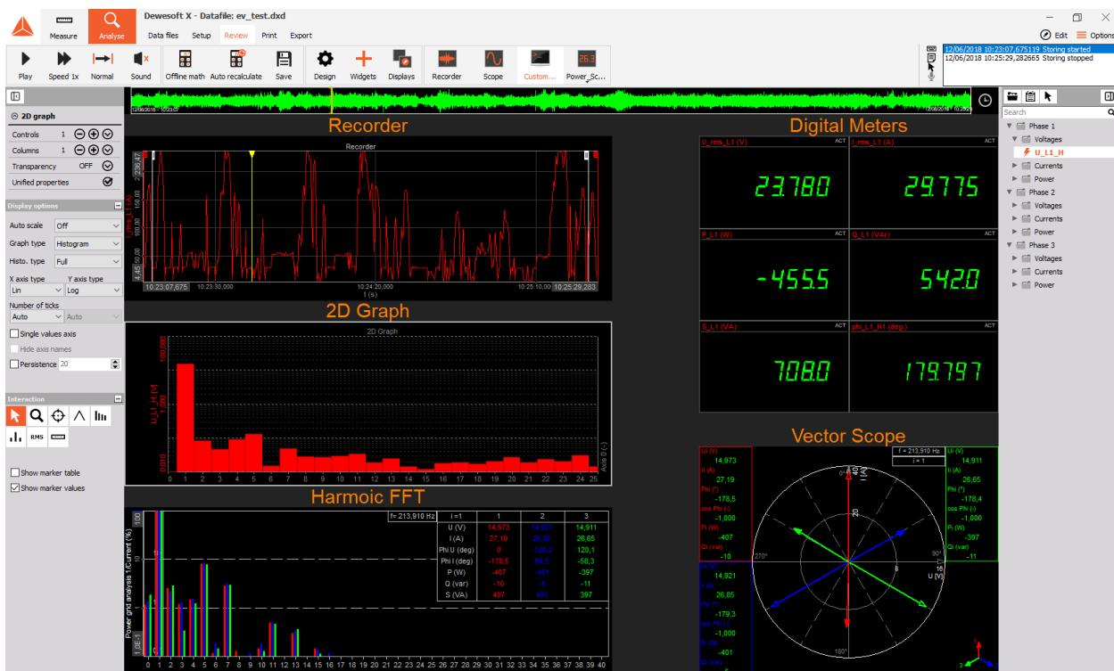
Figure 148. Display options for the measurement screen in the power module
