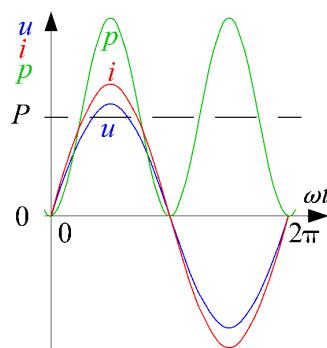
Figure 61. Power calculation graph
