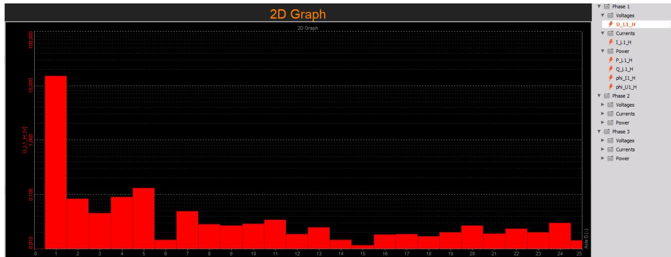
Figure 151. Harmonic 2D graph measurement screen
