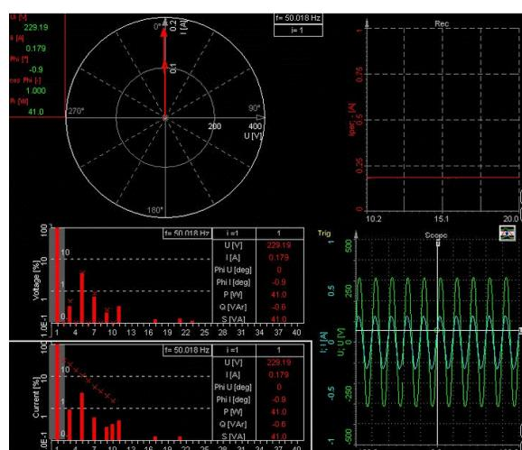
Figure 55. Eliminated phase shift that was caused by the current transducer
