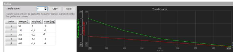
Figure 53. Defining the transfer curve in the analog sensor editor
