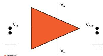
Figure 6. Schematic illustration of a single ended amplifier
