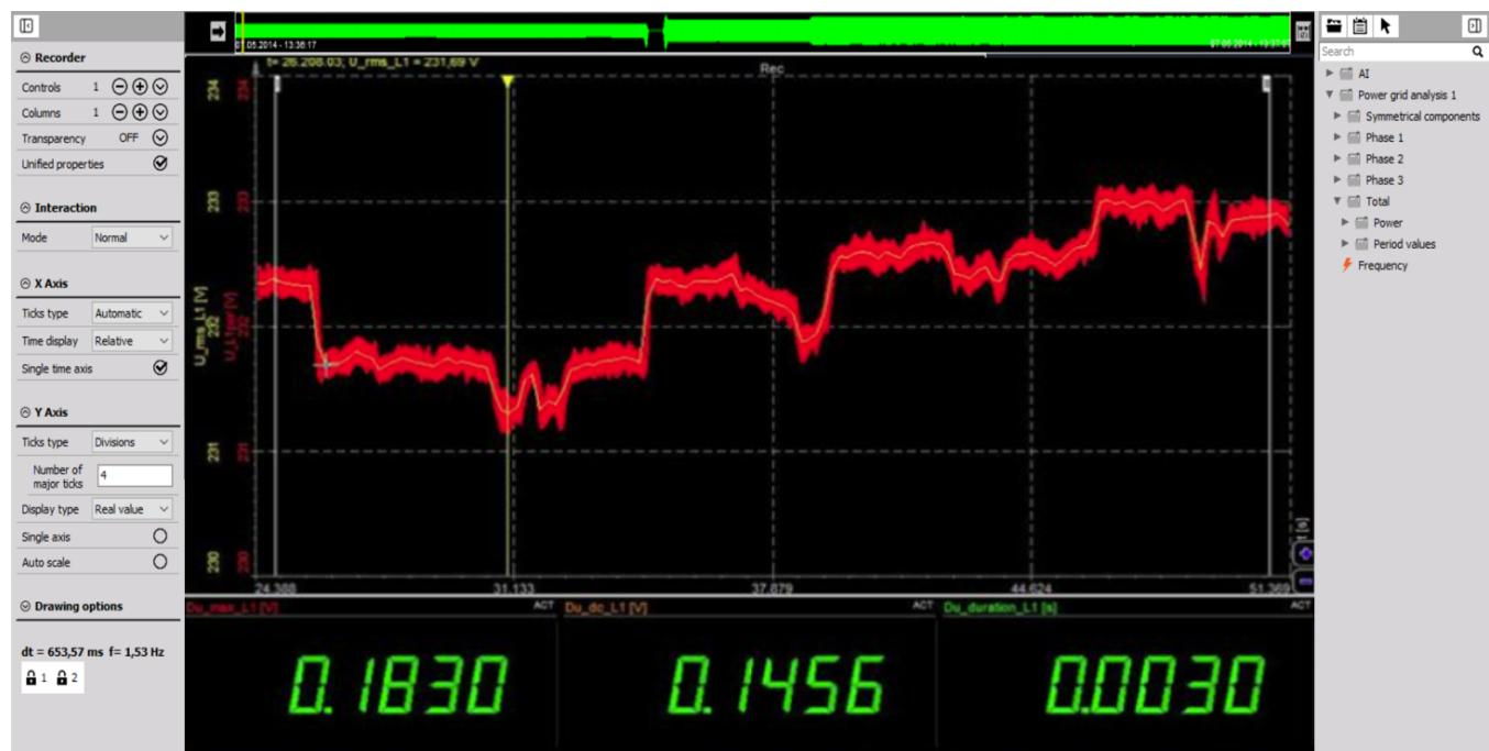
Figure 176. Rapid voltage change measurement screen
