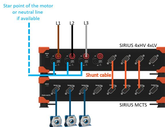
Figure 105. Phase star measurement hardware setup
