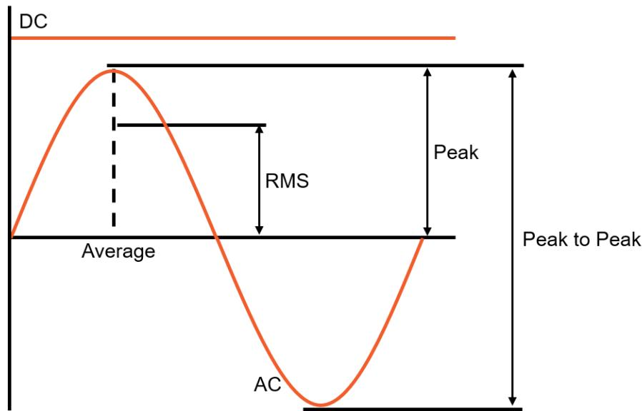
Figure 4. Voltage types: peak, peak-to-peak, average, RMS, AC and DC
