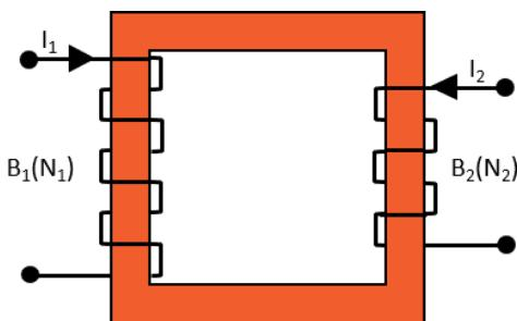
Figure 35. Schematic illustration of the working principle of an iron core clamp
