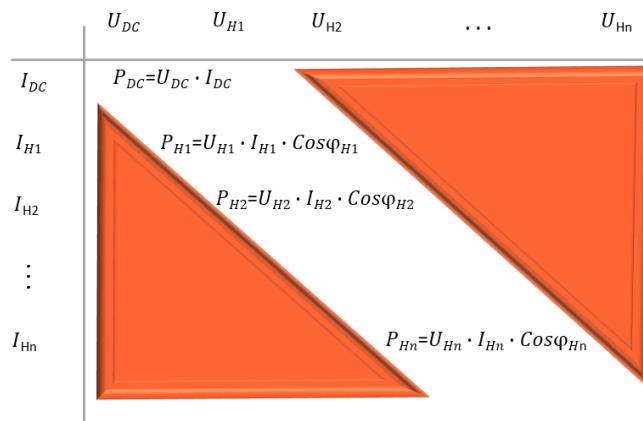
Figure 65. Calculation of harmonic active power values
