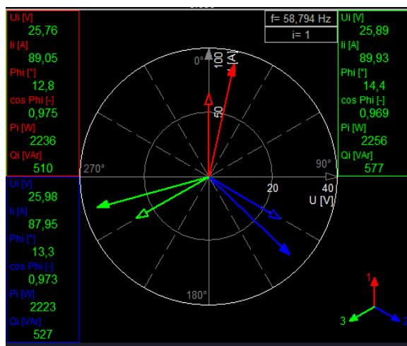
Figure 80. phase vectorscope
