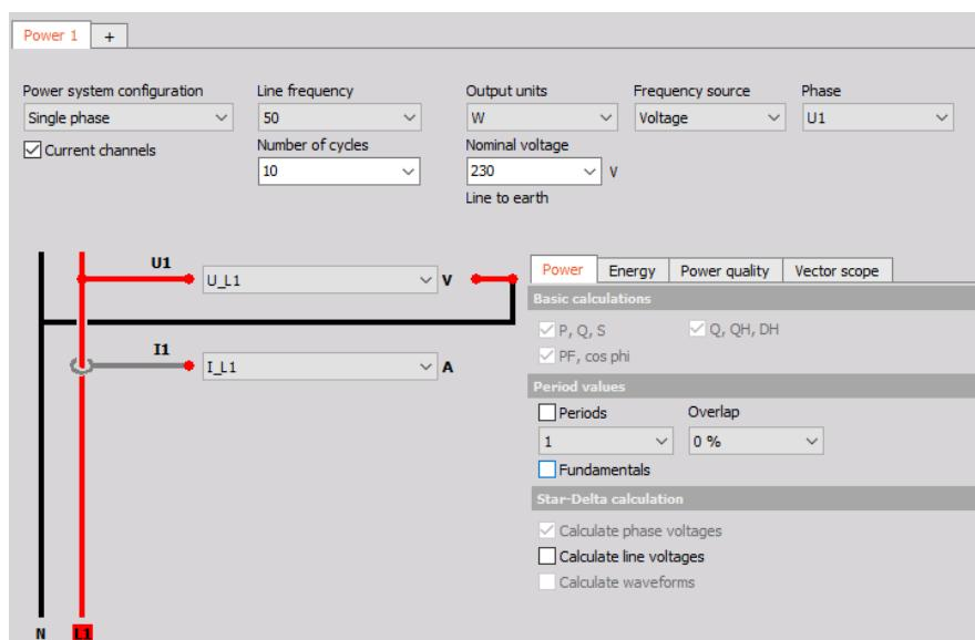
Figure 98. Single phase power module setup screen
