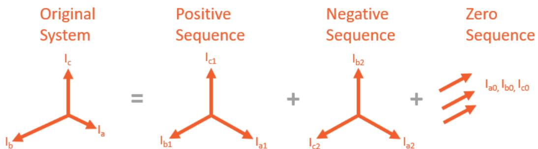
Figure 159. Unbalanced system to balanced system transformation
