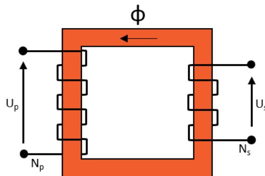
Figure 17. Schematic illustration of the working principle of a voltage transducer
