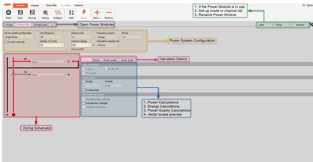
Figure 69. Overview of the power module setup screen
