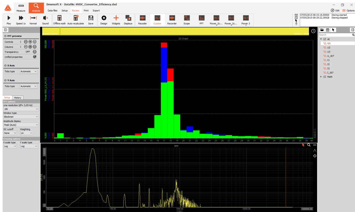
Figure 154. Interharmonic measurement screen in a 2D graph and a FFT graph
