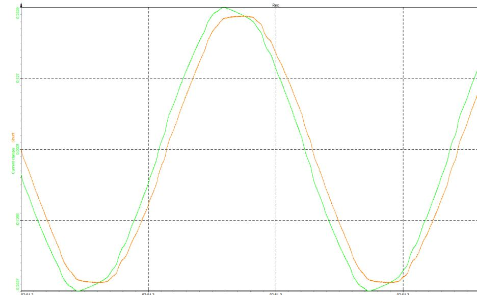
Figure 59. Phase shift between the current clamp and the shunt resistor
