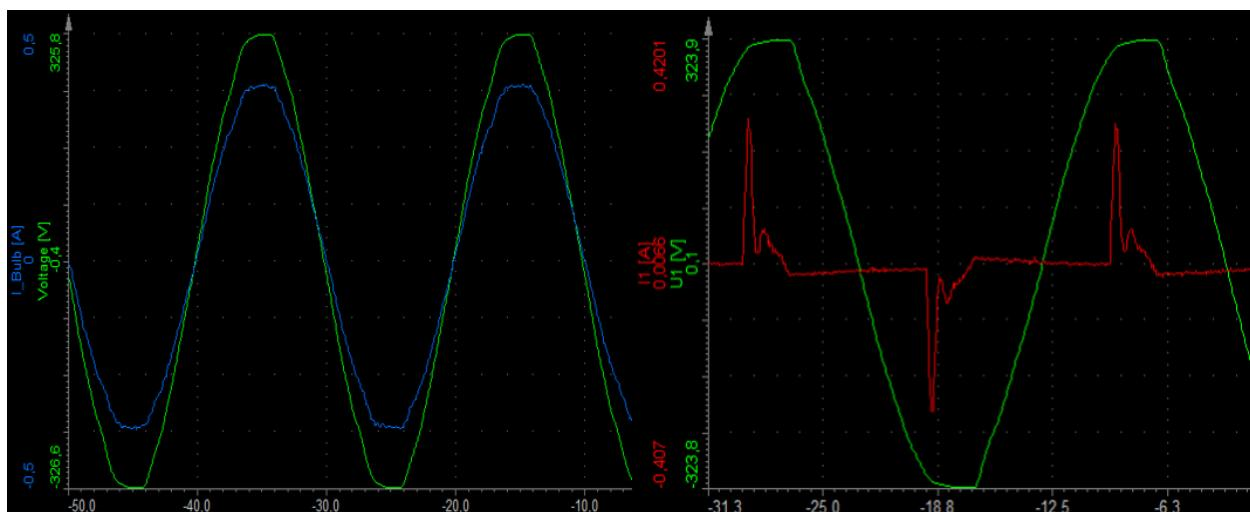
Figure 87. Scope view of a pure ohmic load and a non-linear load
