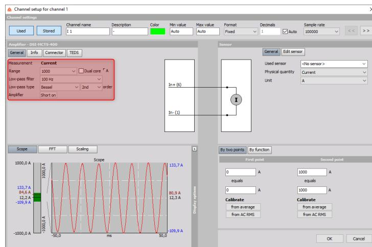
Figure 48. Set up screen for transducers in DewesoftX®
