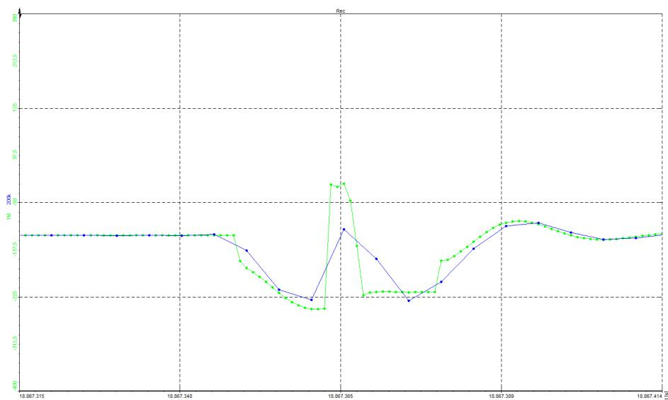
Figure 11. High speed amplifier vs. dual core amplifier transient recording
