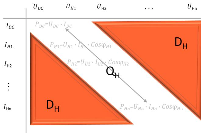
Figure 67. Calculation of harmonic power values for the new power triangle
