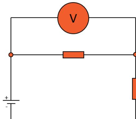
Figure 3. Schematic illustration for connecting a voltmeter
