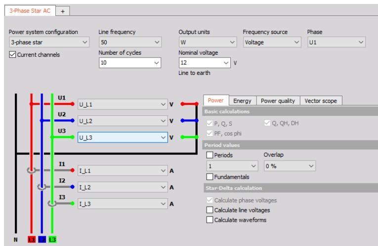
Figure 108. Phase star power module setup
