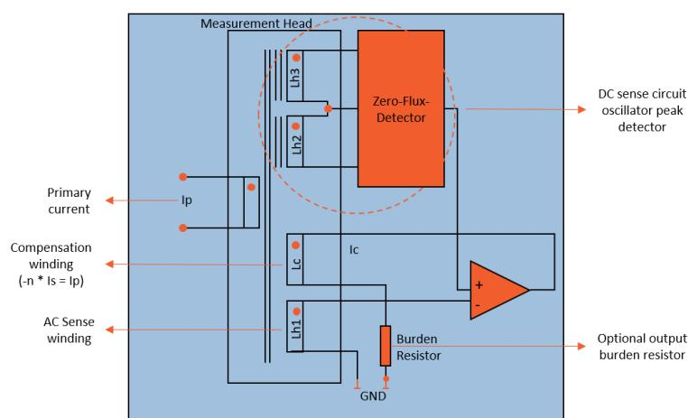
Figure 41. Schematic illustration of the working principle of a Zero-flux transducer
