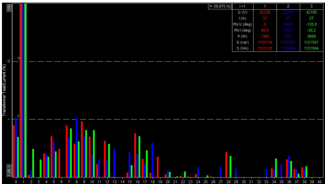
Figure 136. Current harmonic measurement screen
