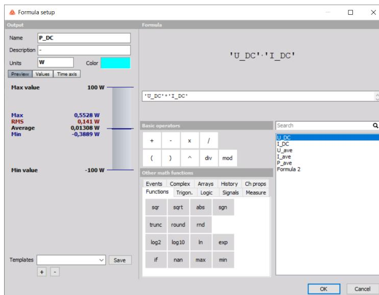
Figure 93. DC math power calculation (only required in Dewesoft X2)
