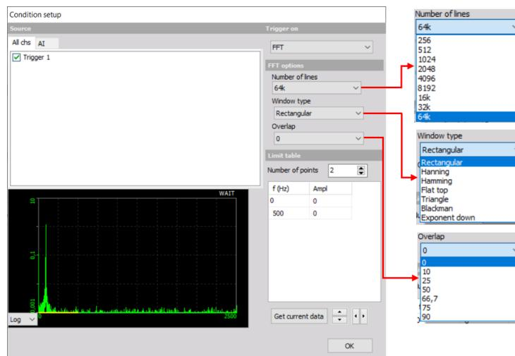
Figure 192. FFT triggering setup
