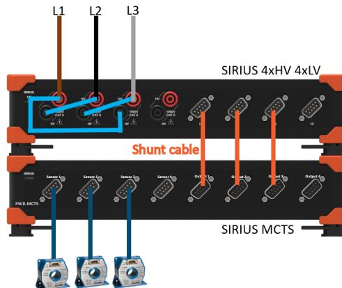
Figure 110. Phase delta measurement hardware setup
