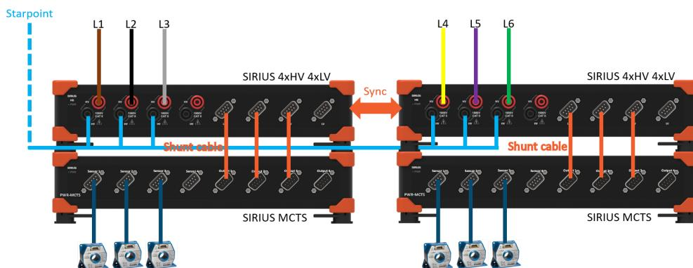
Figure 129. Phase motor measurement setup
