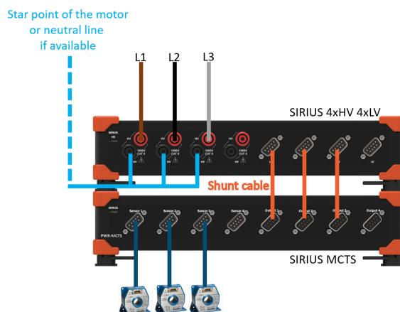
Figure 45. Three phase star point connection with zero-flux transducers
