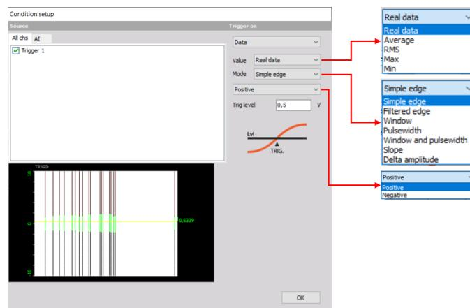
Figure 190. Data triggering setup
