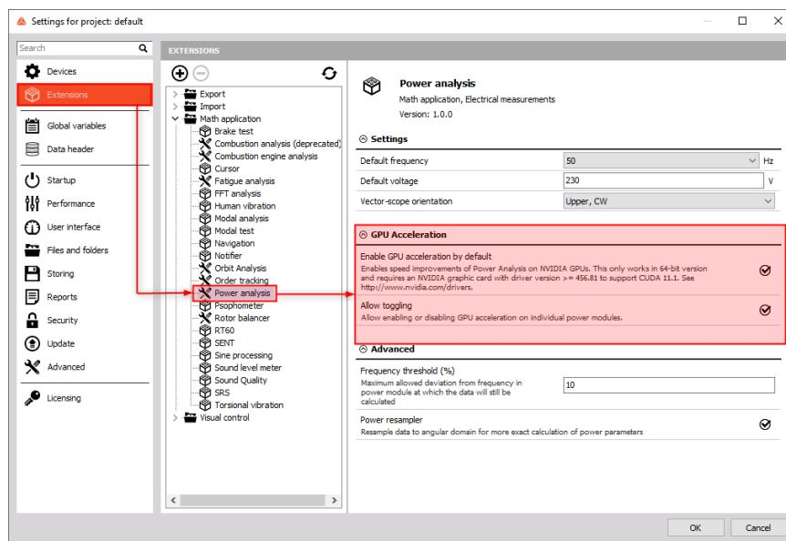
Figure 205. Activating the GPU Acceleration
