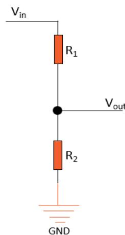
Figure 16. Simple resistor voltage probe with the serial connection of two resistors
