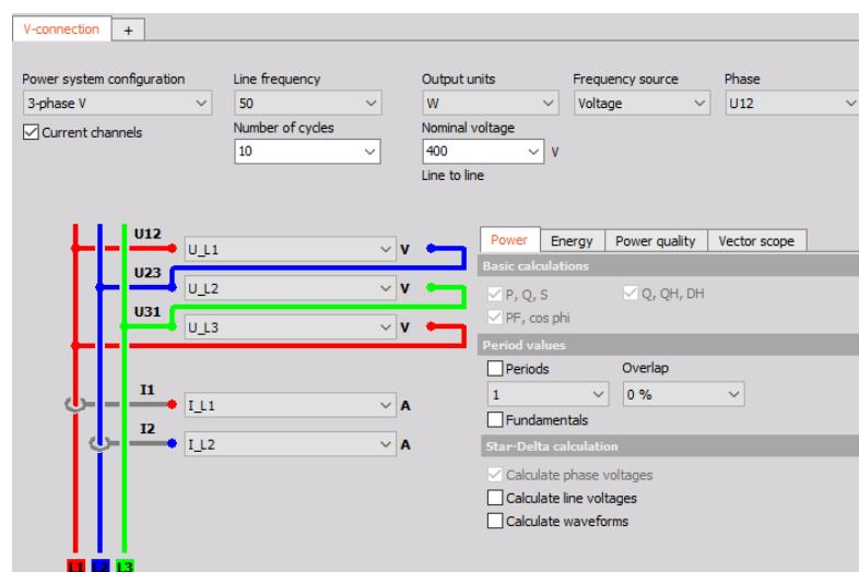
Figure 123. V-connection power module setup
