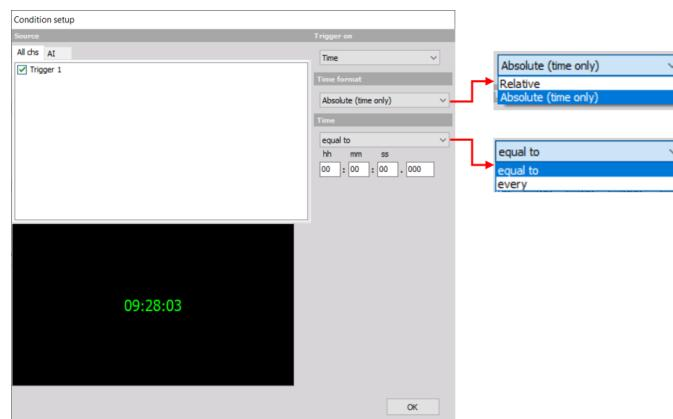
Figure 191. Time triggering setup
