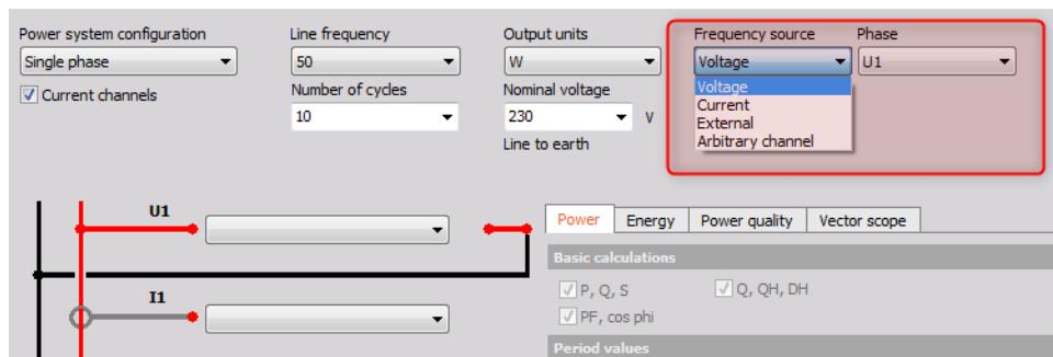
Figure 73. Frequency source in the power module
