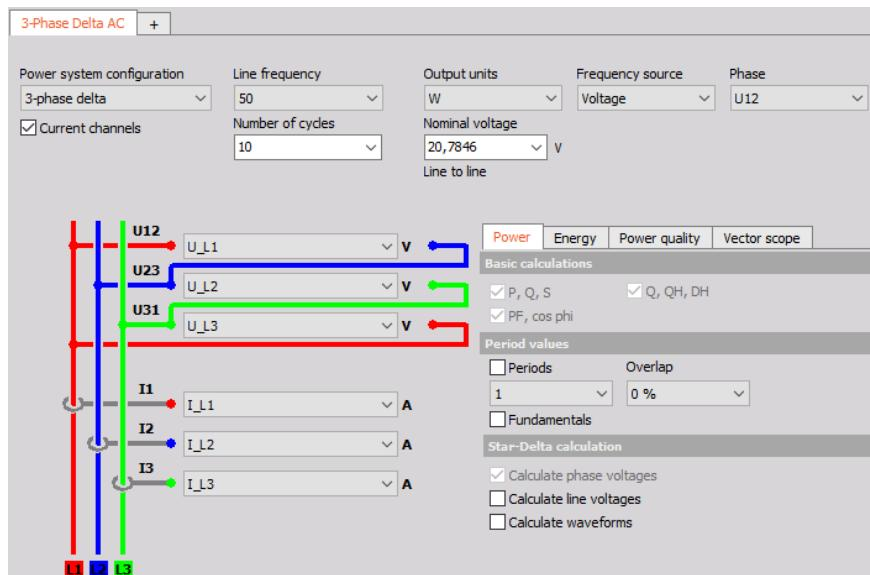
Figure 113. Phase delta power module setup
