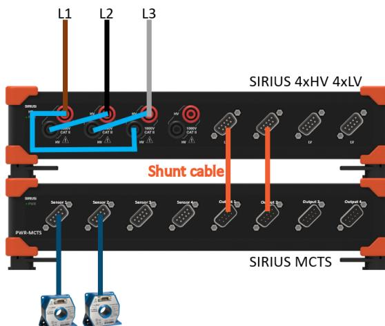
Figure 122. V-connection hardware setup
