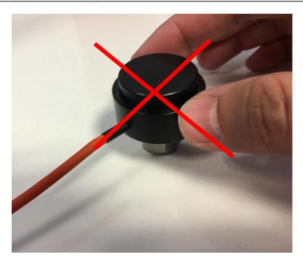
ALWAYS USE A WRENCH AT THE FORCE TRANSDUCER TO REMOVE THE SHAKER FROM THE MOUNTING SURFACE!
