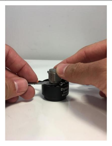
NEVER APPLY FORCE ON THE SHAKER BODY TO REMOVE THE SHAKER FROM THE MOUNTING SURFACE!
