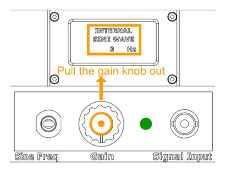
Raise or lower the Sine Frequency Generator Switch to the desired Sine frequency. Adjust the Gain of the amplifier by turning the Gain Knob clockwise. The frequency of the generated sine signal will be visible on the LCD Screen.
