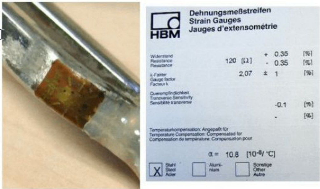
Image 21: Strain gage data
