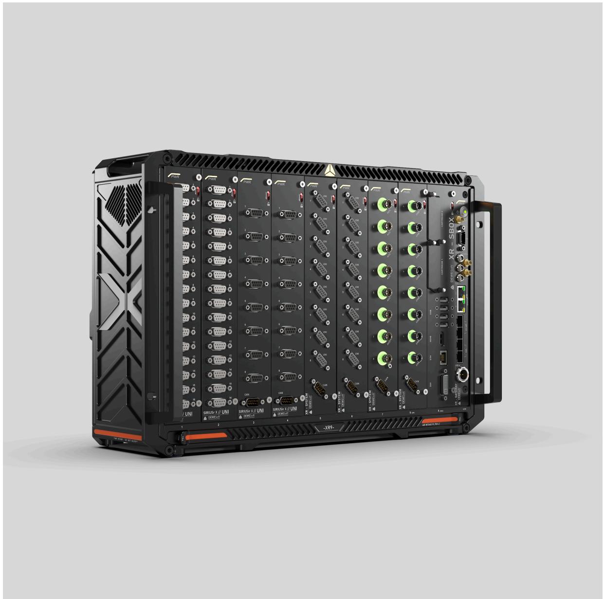
Typical configuration: SIRIUS X 32xUNI, 16xCAN, SIRIUS XHS 16xUNI, 8xACC, 8xCHG, XR-SBOX
